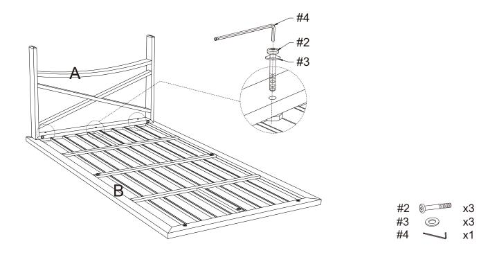
Step 2. Attach rails (part C) to side panel (part A) and top panel (part B) using short bolts (part #1), flat washers (part #3) and allen wrench (part #4).
