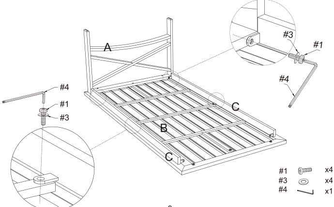
Step 3. Attach side panel (part A) to top panel (part B) and rails (part C) using short bolts (part #1), long bolts (part #2), flat washers (part #3) and allen wrench (part #4).
